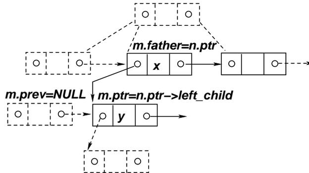
Figura 3.22: La función `lchild()`.
